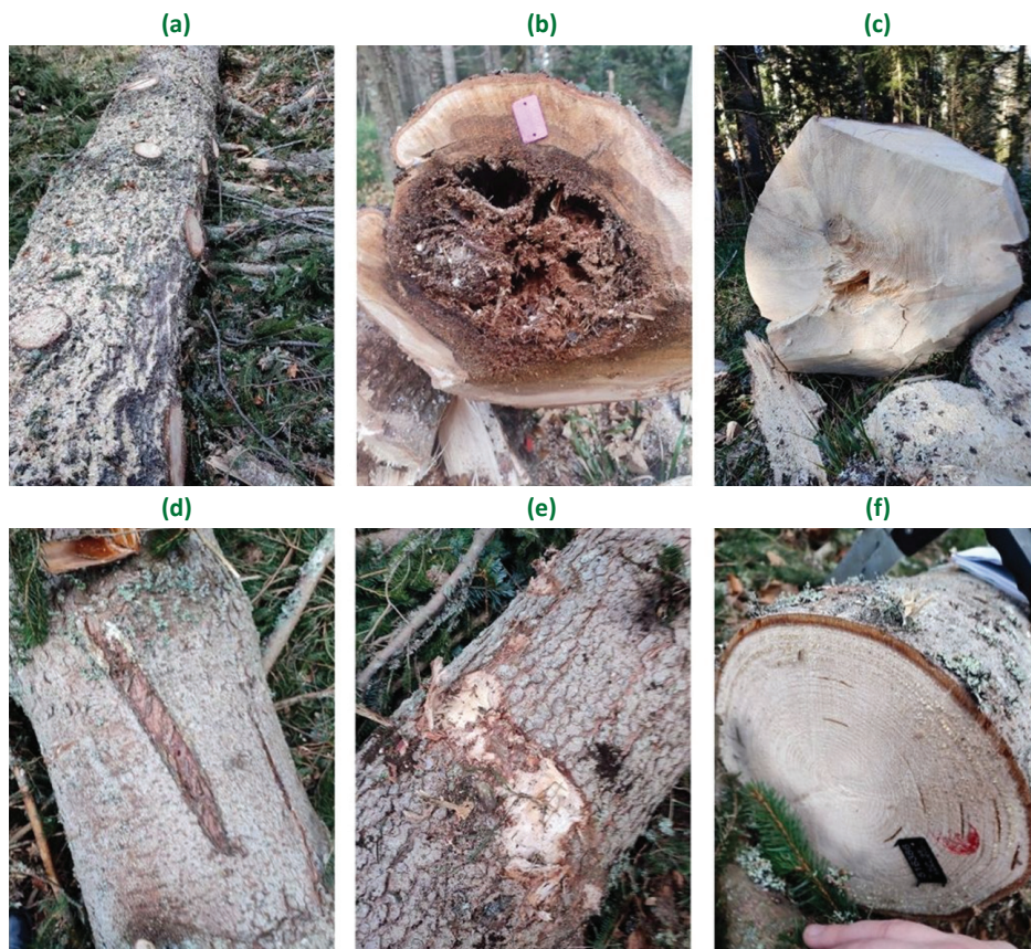
Figure 2. Some of the recorded wood defects in Norway spruce. (a) knots; (b) rot; (c) pith eccentricity and compression wood; (d) scar; (e) damage caused by mechanical factor; (f) resin pockets.
